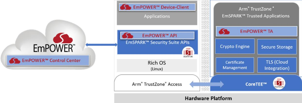
**Figure 1 Cloud – Device Components**
